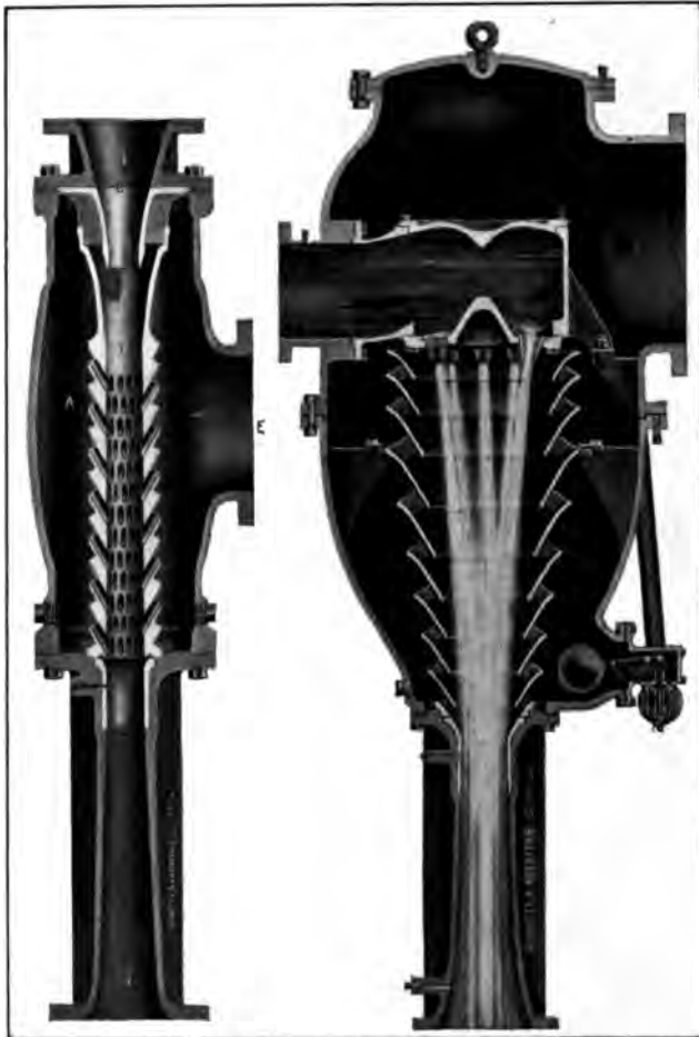
FIG. 52.—Koerting eductor and multijet condensers.
